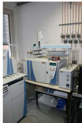
DeltaV with EA, GC-Isolink and Precon => currently mainly N 2 O isotopes from lab and field studies
